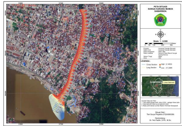
Gambar 4. Peta Situasi Batimetri (Jalur Long Section dan Cross Section) Figure 4. Bathymetric Situation Map (Long-Section and Cross-Section Lines)
